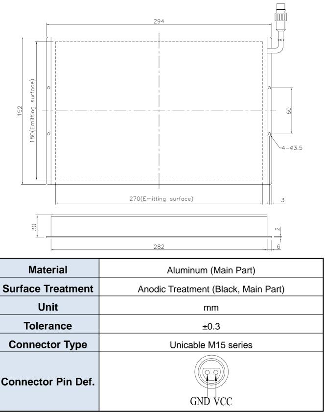
Note: Owing to the different series of lights, the length of wires is about 25 - 30cm.
