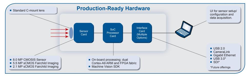
MityCAM is Critical Link's family of highly configurable imaging and vision solutions. The platform is designed to be customizable with a variety of high-performance sensors, user programmable SoC featuring tightly integrated ARM and FPGA fabric, and multiple I/O options. Customers benefit from the platform's flexibility, with each building block tailorable to suit the application.
