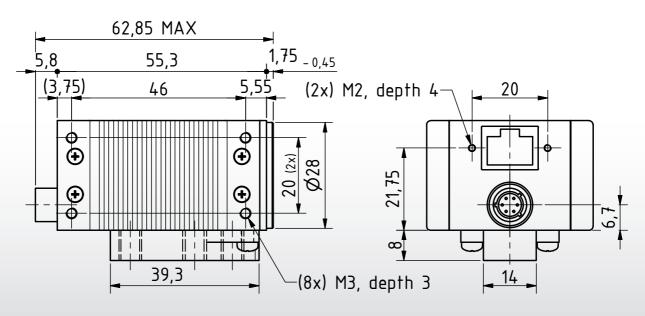
Dimensions: mm Tolerances: DIN ISO 2768m
