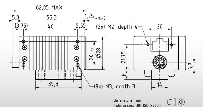
Dimensions: mm Tolerances: DIN ISO 2768m
