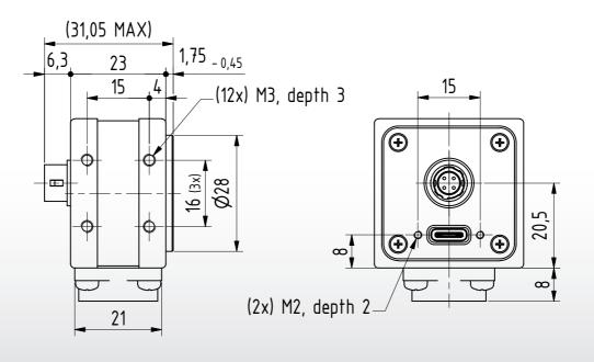
Dimensions: mm  $\Box \oplus$ Tolerances: DIN ISO 2768-f
