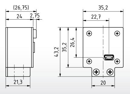
Dimensions: mm Tolerances: DIN ISO 2768m
