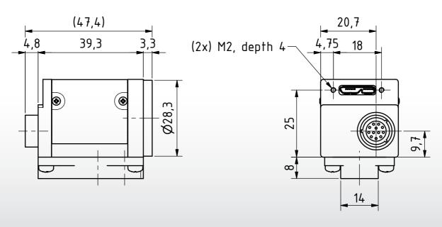
Dimensions: mm Tolerances: DIN ISO 2768m
