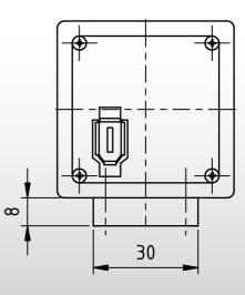
Dimensions: mm Tolerances: DIN ISO 2768m
