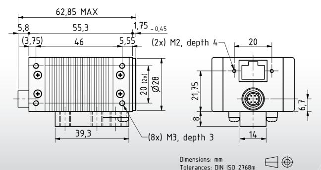
Dimensions: mm Tolerances: DIN ISO 2768m
