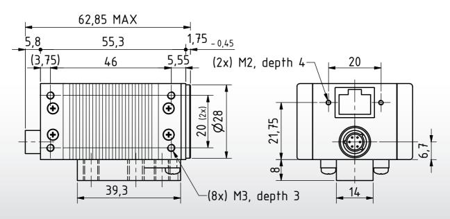
Dimensions: mm Tolerances: DIN ISO 2768m
