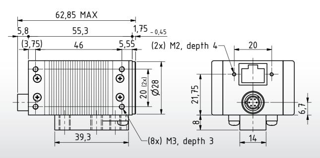
Dimensions: mm Tolerances: DIN ISO 2768m
