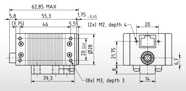
Dimensions: mm Tolerances: DIN ISO 2768m
