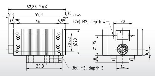
Dimensions: mm Tolerances: DIN ISO 2768m
