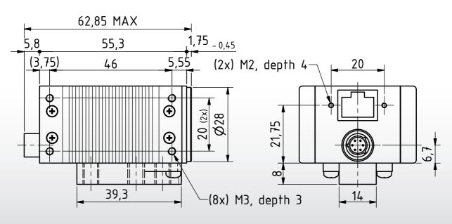
Dimensions: mm Tolerances: DIN ISO 2768m
