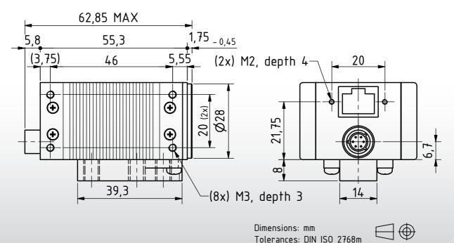
Dimensions: mm Tolerances: DIN ISO 2768m
