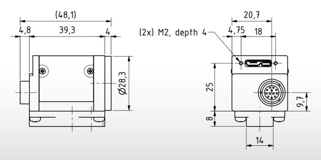
Dimensions: mm Tolerances: DIN ISO 2768m
