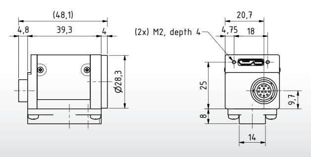
Dimensions: mm Tolerances: DIN ISO 2768m
