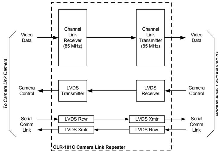
Figure 1-1: CLR-101C Block Diagram
