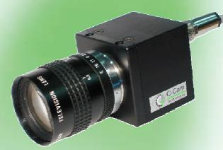
The BCi5 camera is a very compact, high-resolution CMOS camera. The camera is equipped with the Ibis5a image sensor with 6.7 µm square pixels. The user can define any Window Of Interest within a 1280 x 1024 pixel area, also known as the SXGA format. The sensor has a remarkably good signal-to-noise ratio in combination with excellent contrast performance
