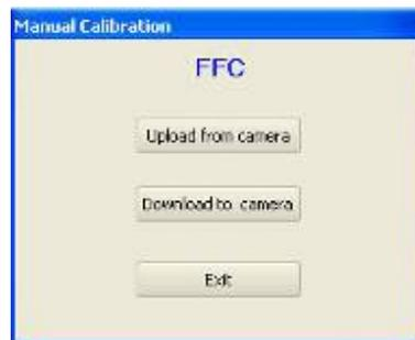
This will allow the user to upload/download out/in the Camera the FFC coefficients in/from a text file that can be processed externally.
