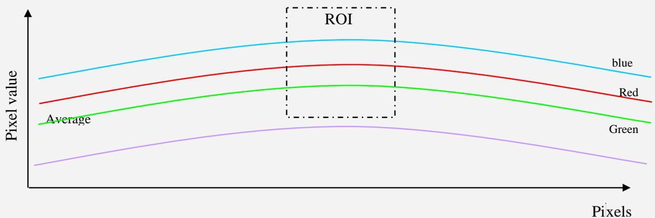
Each gain is then calculated to reach the level of the color which has the highest sensitivity.
