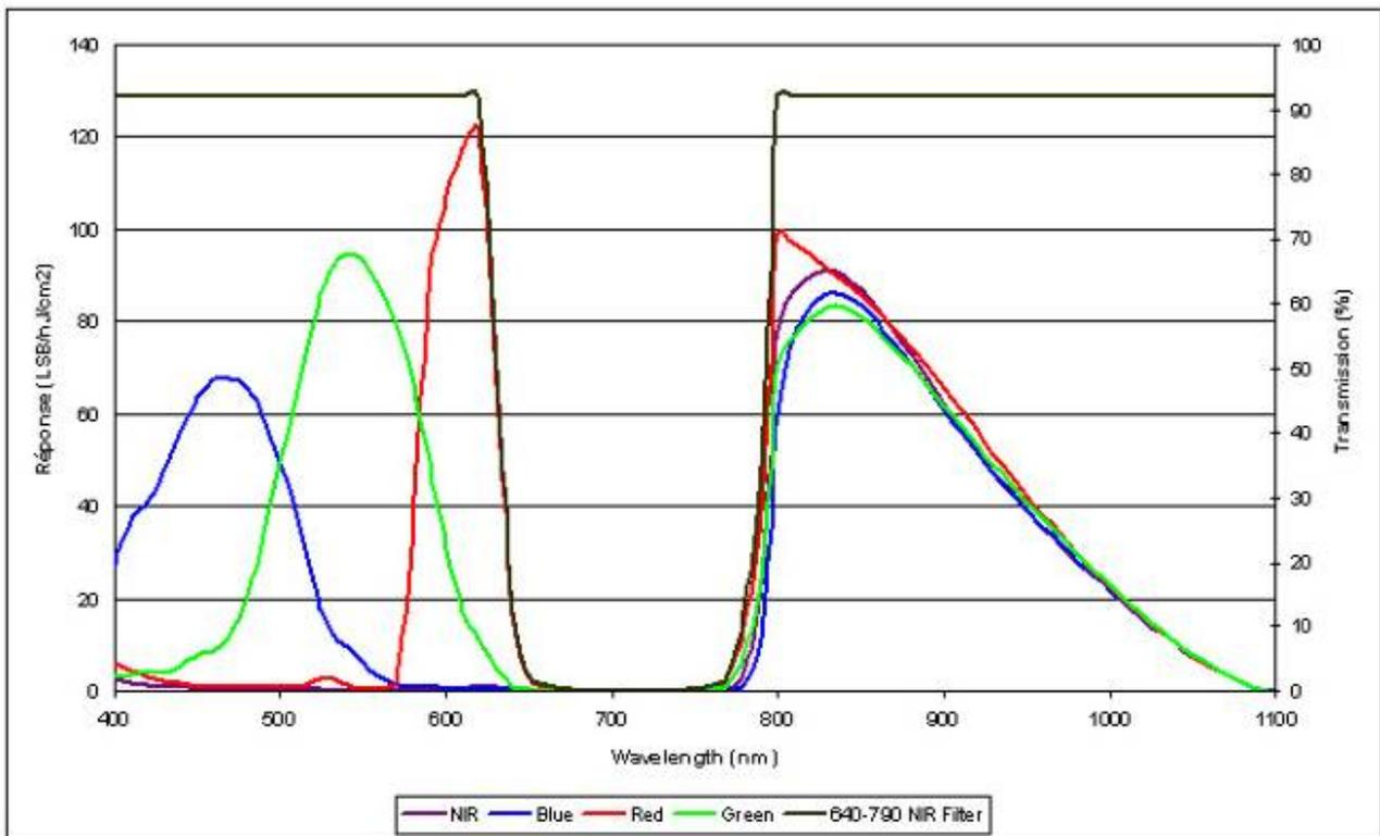
The sensor has been designed to give in the Near Infra Red (800-1100nm) an equal answer of each Red, Green and Blue colors than the Nir line itself.
