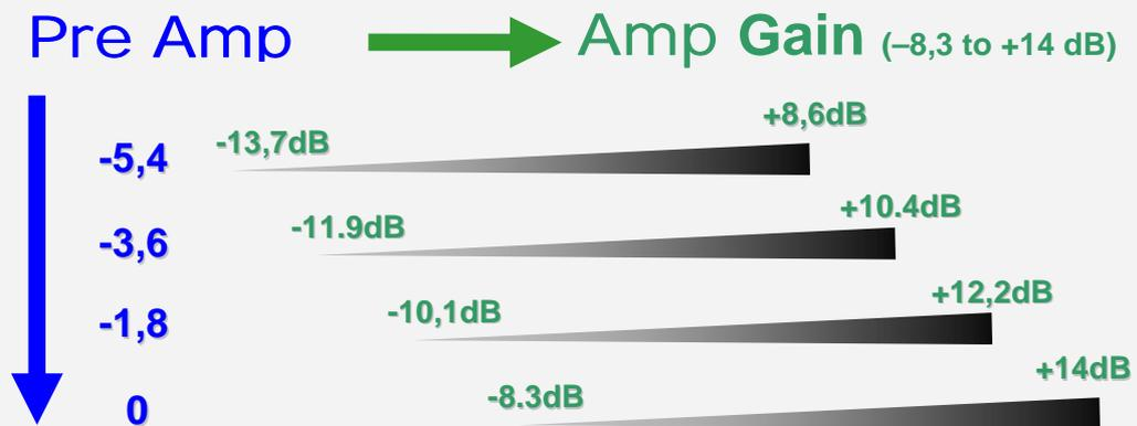
⇒ The best tuning is when the Amplification Gain is at its minimum possible
