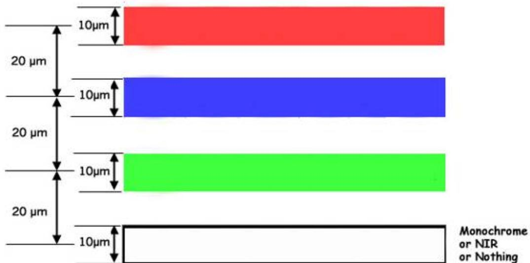
**Note:** The real order of the color line is Red-Blue-Green but the Camera outputs in Red-Green-Blue order on the Camera Link connector.
