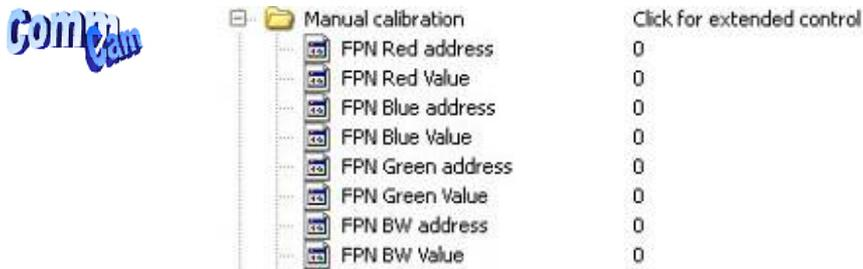
⇒ Read function : "**r ffco <addr> <nbrval> [crcreq]**": Read <nbrval> FPN user coefficients starting from <addr> address. If [crcreq] is equal to 1, the crc will be calculated on the outputted value.
