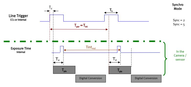
In these modes, the rising edge of the Trigger (internal or External) starts the readout process  $(T_{pix})$  of the previous integration. The Real exposure time (Tint<sub>real</sub>) is finally equal to the Line Period  $(T_{per})$  even if it's delayed from  $(T_x + T_d)$  from the rising edge of the incoming Line Trigger.
