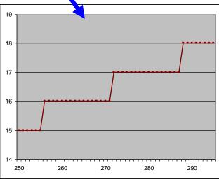
An increment of 1 LSB is made every 16 pixels When it reaches 255, turns back to 0 and starts again
