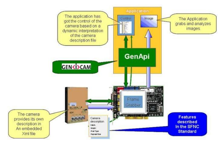
The Frame Grabber software is supposed to propose a feature Brother, based on GenlCam, which lists and allows the modification of the parameters of the Camera.
