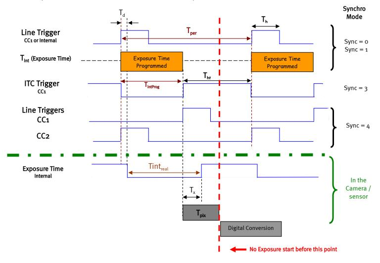
$T_{pix}$ : Timing Pixel. During this uncompressible period, the pixel and its black reference are read out to the Digital converter. During the first half of this timing pixel (read out of the black reference), we can consider that the exposure is still active.
