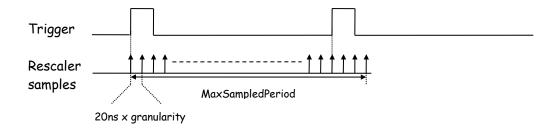
The MaxSampledPeriod must be as close as possible to the trigger period while still being longer MaxSampledPeriod =  $2 \text{ons } x \text{ granularity } x 2^{\text{rescalerSize}}$
