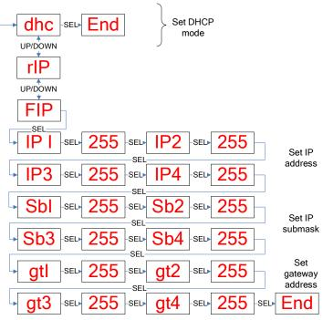
When an IP address has been assigned using DHCP, the address can be read from the keypad as follows. Press and hold the SEL button until the display shows "OP1". Use the UP and DOWN buttons to select "ETH" then press SEL. Use the UP and DOWN buttons to select "rIP" and press SEL. Keep pressing SEL and read the four values of the IP address. The example below shows the IP address 192.168.1.71.
