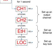
either be done with the KB Ethernet command or from the keypad. A lock code is used. Users who know the lock code can unlock the keypad. The lock code is from 0 to 255, providing moderate protection.
