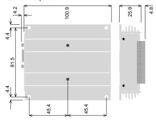
The PP500 can be mounted from above using the M4 clearance corner holes, or from beneath using the M4 tapped holes (maximum screw length inside is 6mm).
