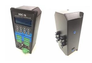
Metaphase Technologies' 16-Channel Quantum Controller (QC-16) provides 0-10VDC intensity control for sixteen independent LED loads in increments of .01V.
