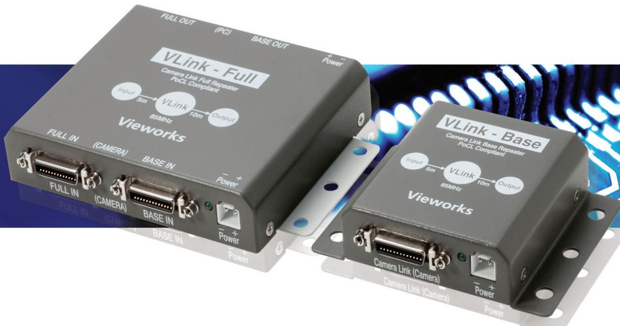
VLink Series is a cost-effective Camera Link repeater to dramatically increase the distance between a camera and frame grabber. It amplifies video signals that are attenuated on the Camera Link cable and doubles the available cable length through LVDS output connector equipped with a pre-emphasis feature. VLink Series allows not only to simplify the machine vision systems but also to save the cost with the least number of the repeaters and cables.
