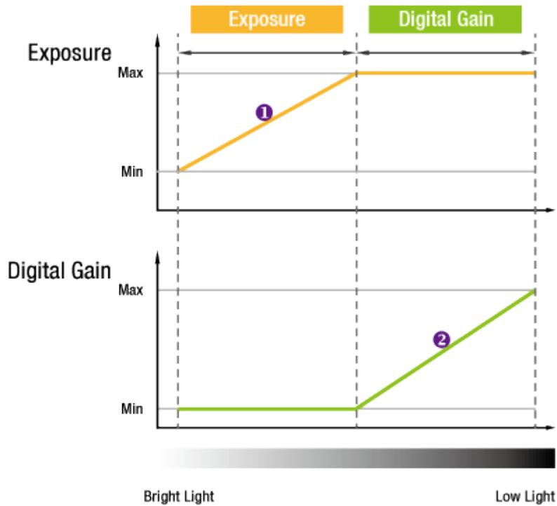
Figure 10.21 Image Level Adjustment
