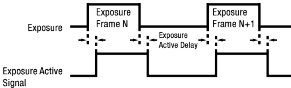
**Figure 10.29 Exposure Active Signal**
