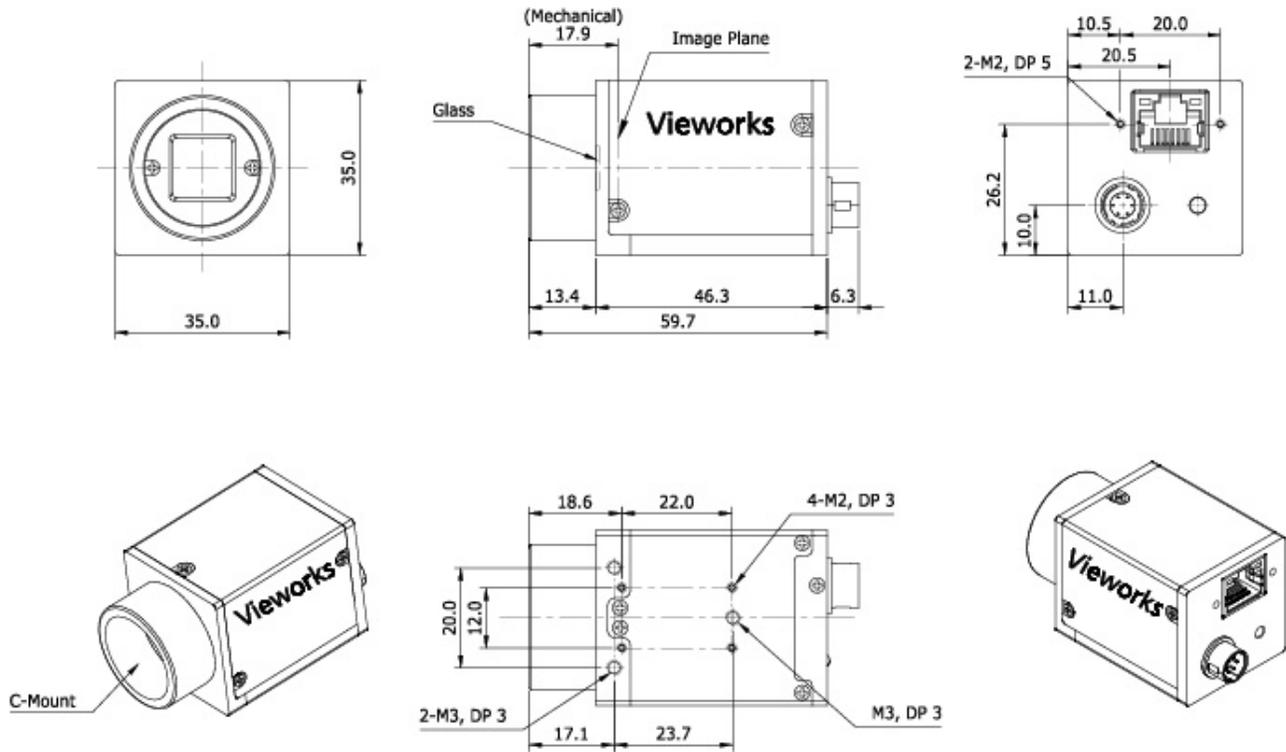
Figure 5.14 VQ-5MG-16 C-mount Mechanical Dimension
