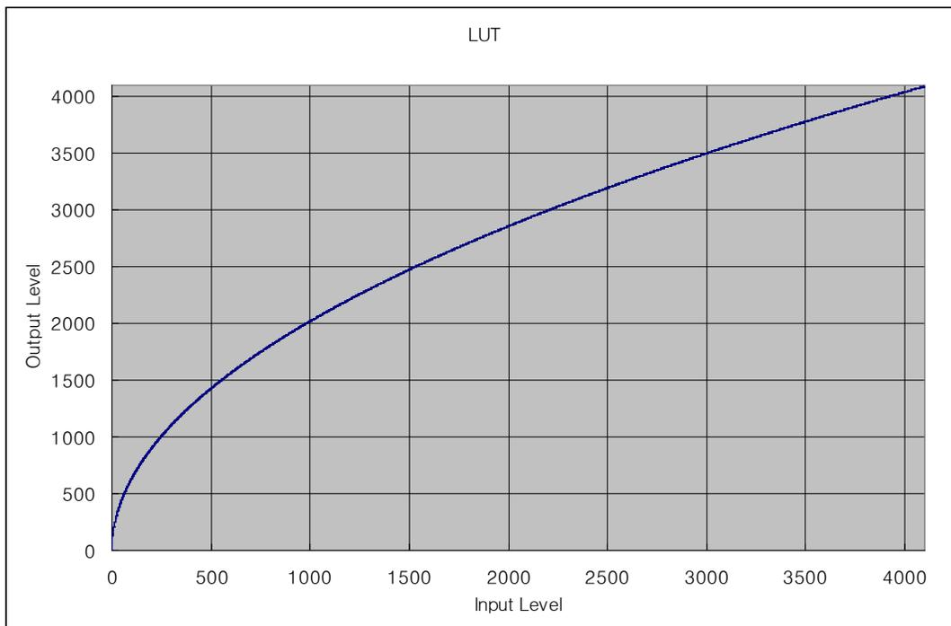
Figure 10.24 LUT at Gamma 0.5
