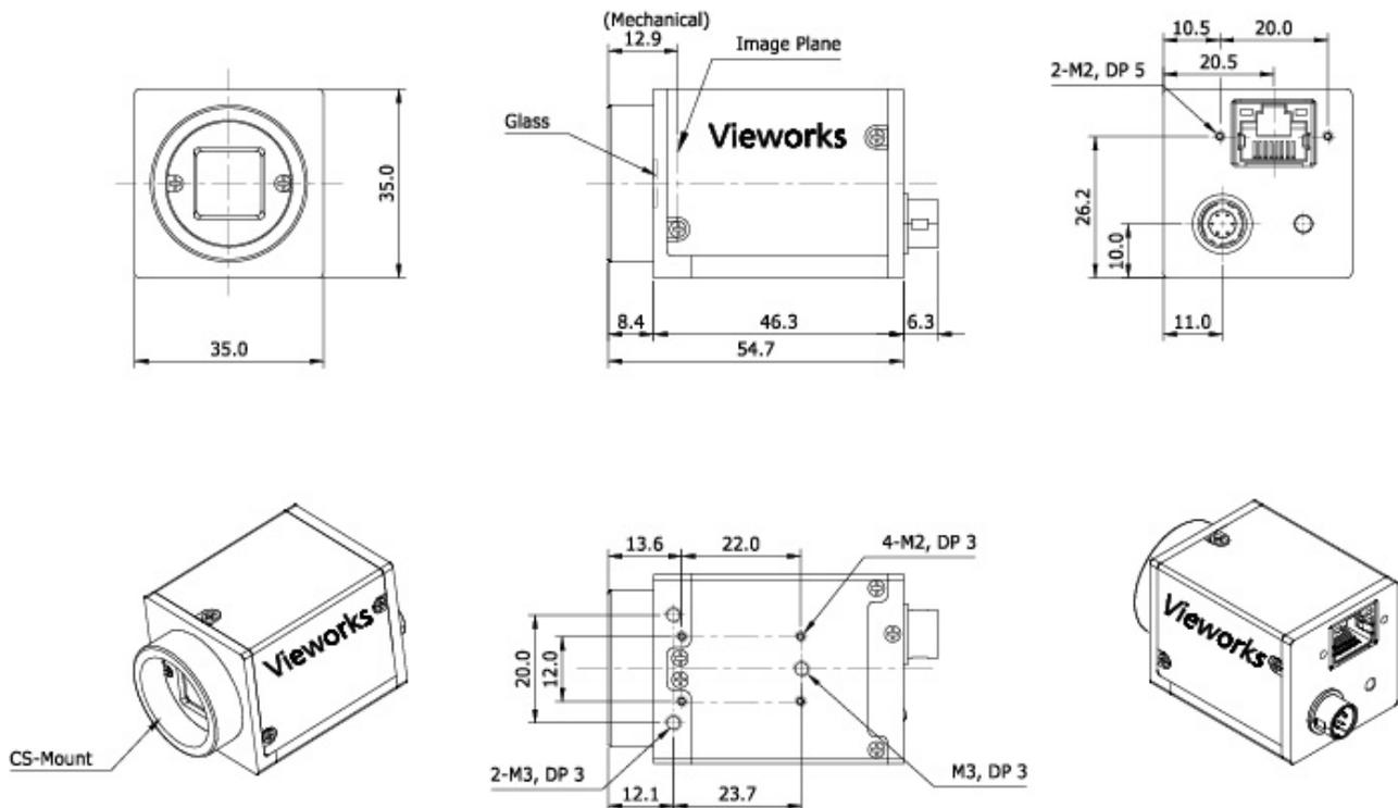
Figure 5.15 VQ-5MG-16 CS-mount Mechanical Dimension
