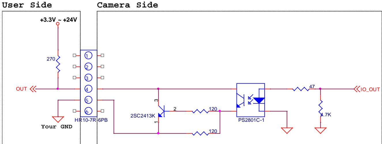
Figure 8.8 I/O Output Schematic
