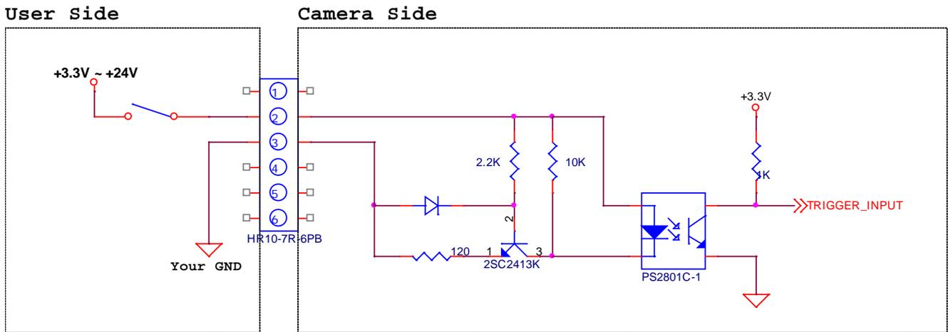
Figure 8.6 Trigger Input Schematic
