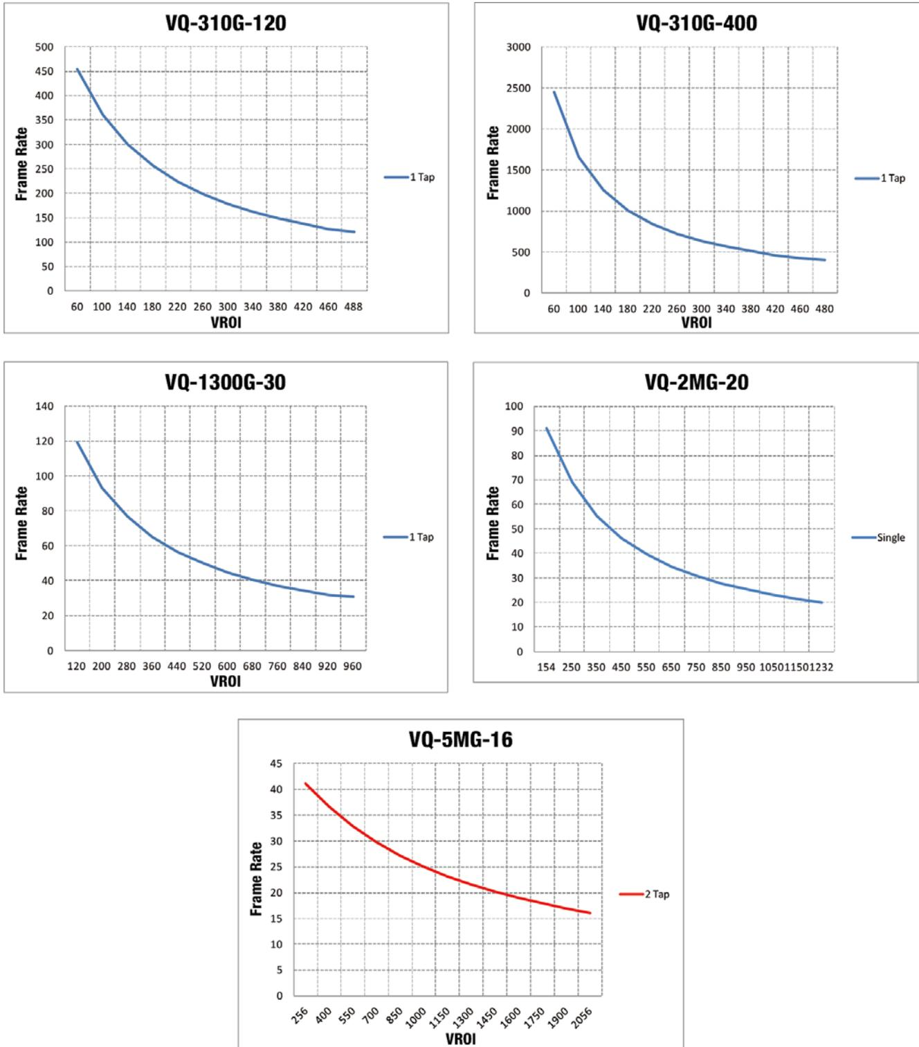
Figure 10.2 Frame Rate by Vertical ROI changes
