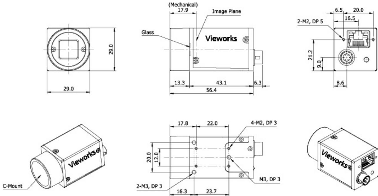
Figure 5.12 VQ-310G-120, 1300G-30 and 2MG-20 C-mount Mechanical Dimension
