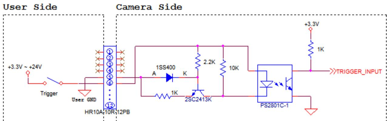
Figure 8.7 Trigger Input Schematic (VQ-310G-M400)
