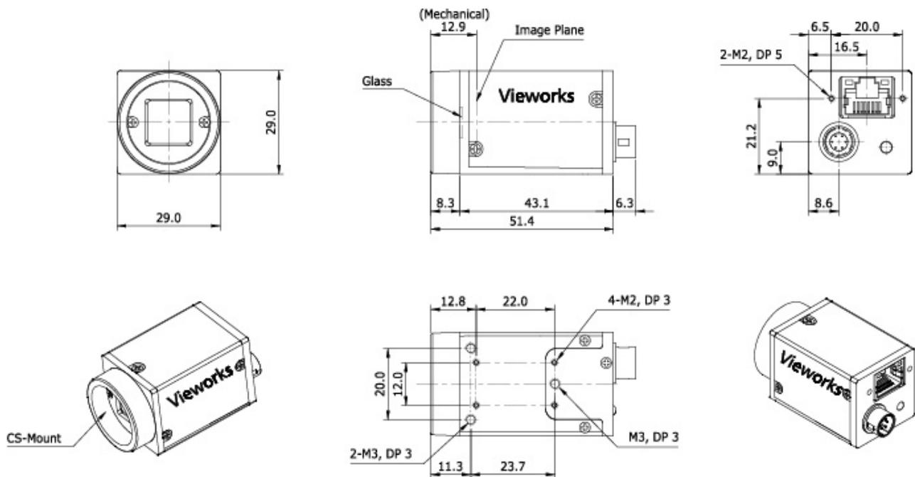
Figure 5.13 VQ-310G-120, 1300G-30 and 2MG-20 CS-mount Mechanical Dimension
