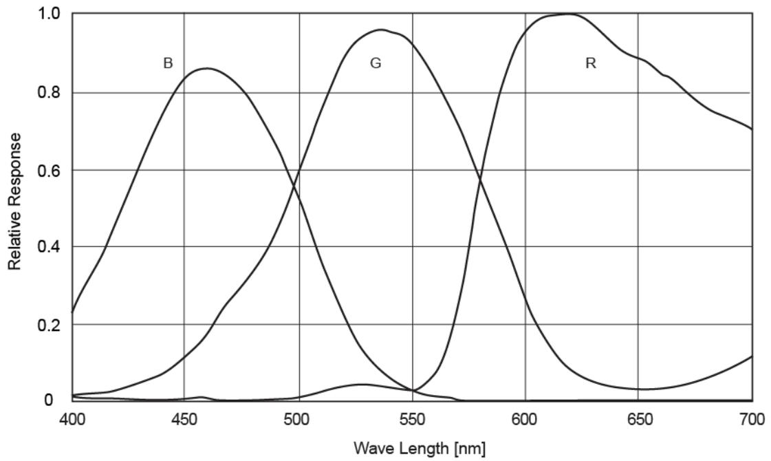
Figure 5.10 VQ-2MG-C20 Spectral Response
