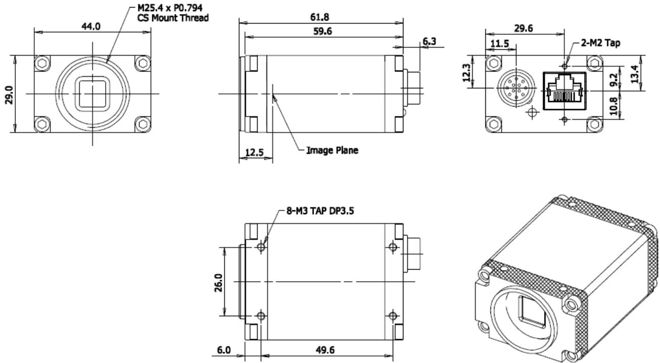
Figure 5.16 VQ-310G-M400 CS-mount Mechanical Dimension
