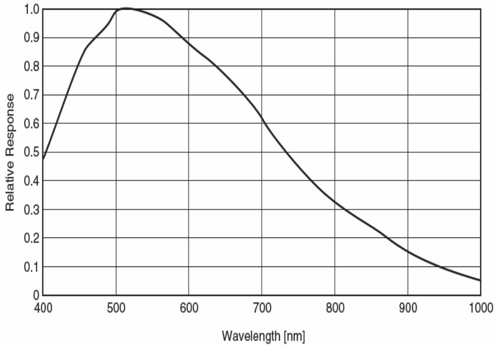
Figure 5.6 VQ-5MG-M16 Spectral Response
