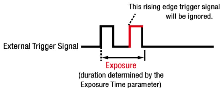
Figure 9.4 Trigger Overlapped with Timed Exposure Mode
