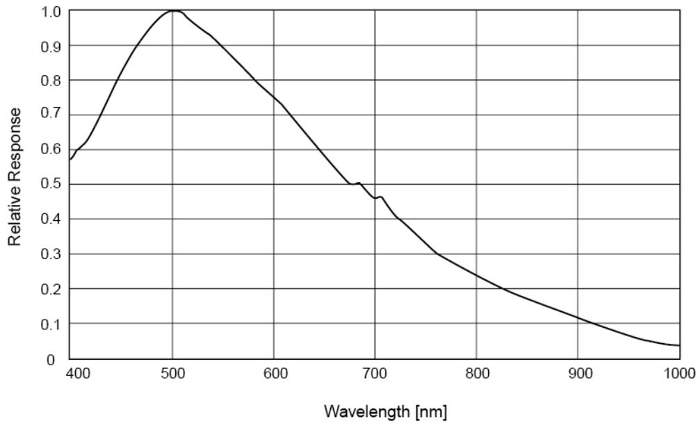
**Figure 5.5 VQ-2MG-M20 Spectral Response**
