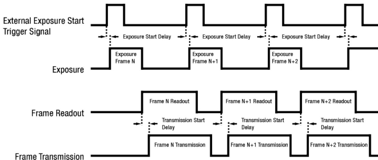
Figure 9.14 Timing Chart (not drawn to scale)
