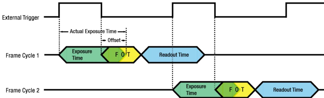
Figure 9.12 Trigger Width Exposure Mode for VQ-310G-M400
