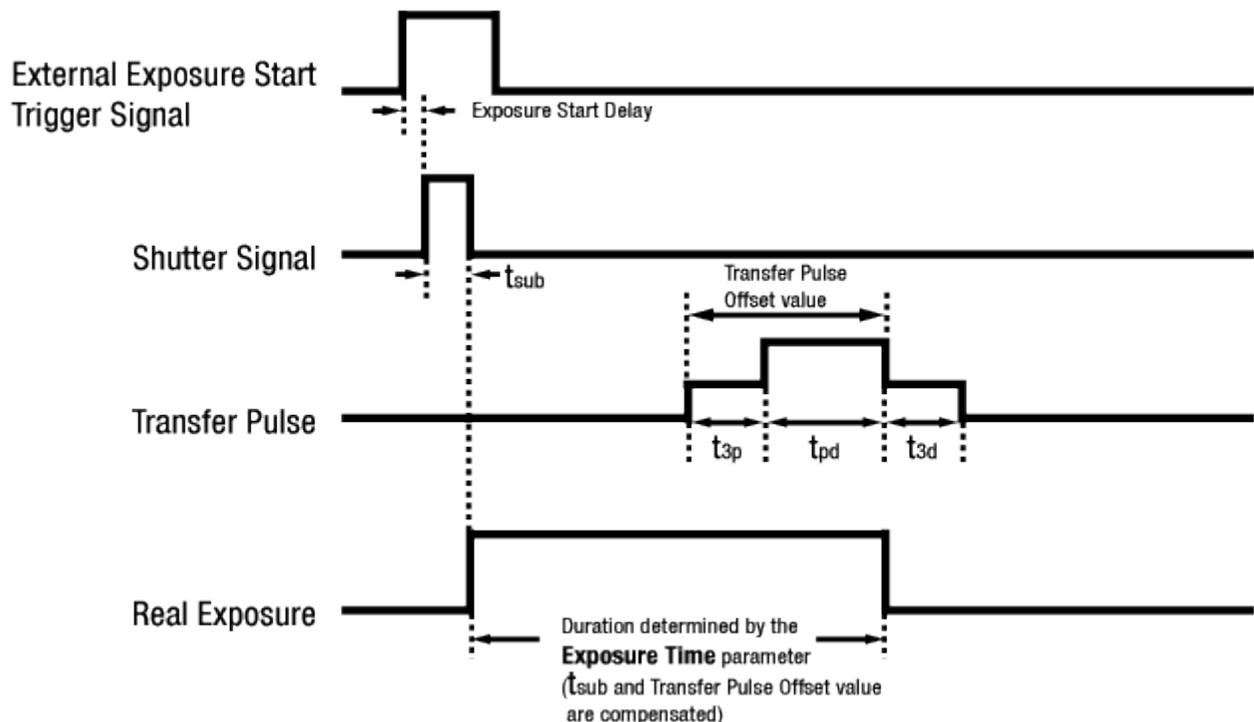
Figure 9.9 Real Exposure with Timed Exposure Mode
