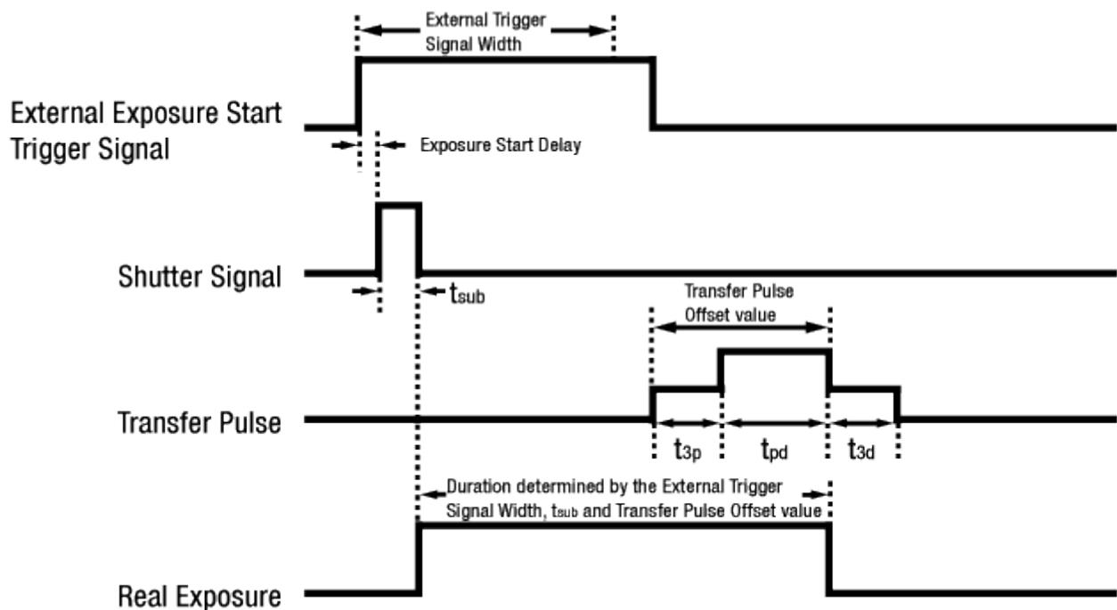
Figure 9.10 Real Exposure with Trigger Width Exposure Mode
