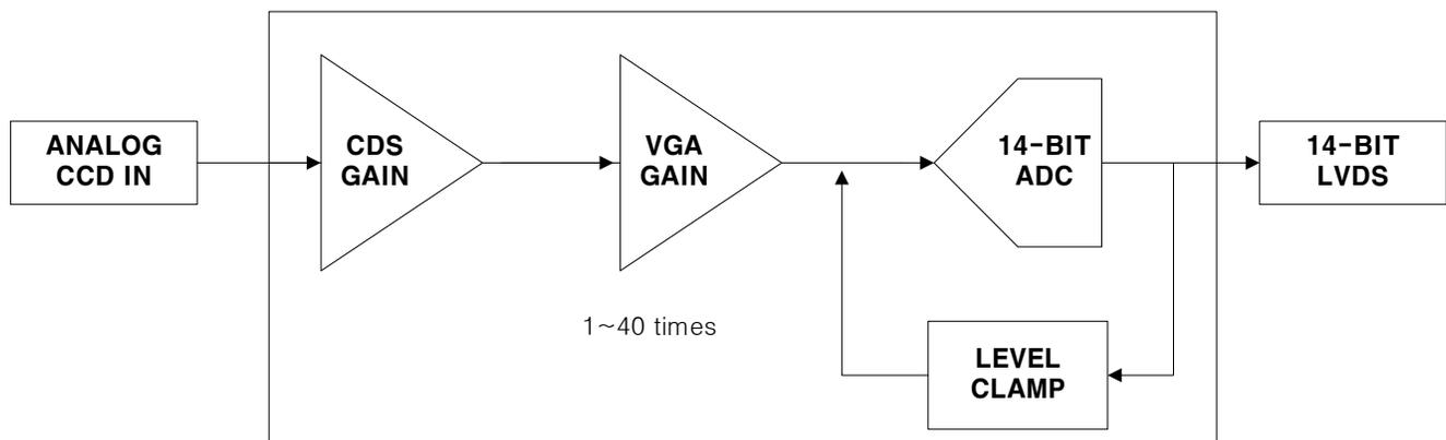
Figure 10.22 AFE Block Diagram
