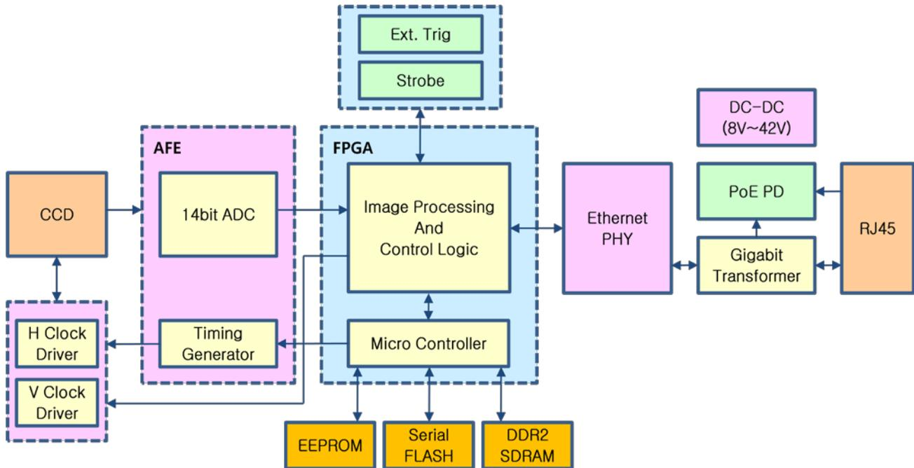
**Figure 5.1 Camera Block Diagram (Except VQ-310G-M400)**
