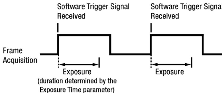
**Figure 9.2 Frame Acquisition with Software Trigger Signal**
