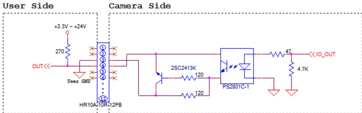
Figure 8.9 I/O Output Schematic (VQ-310G-M400)
