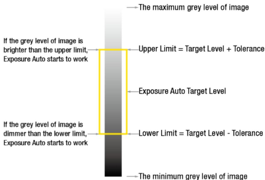
Figure 10.20 Exposure Auto Target Level and Exposure Auto Tolerance
