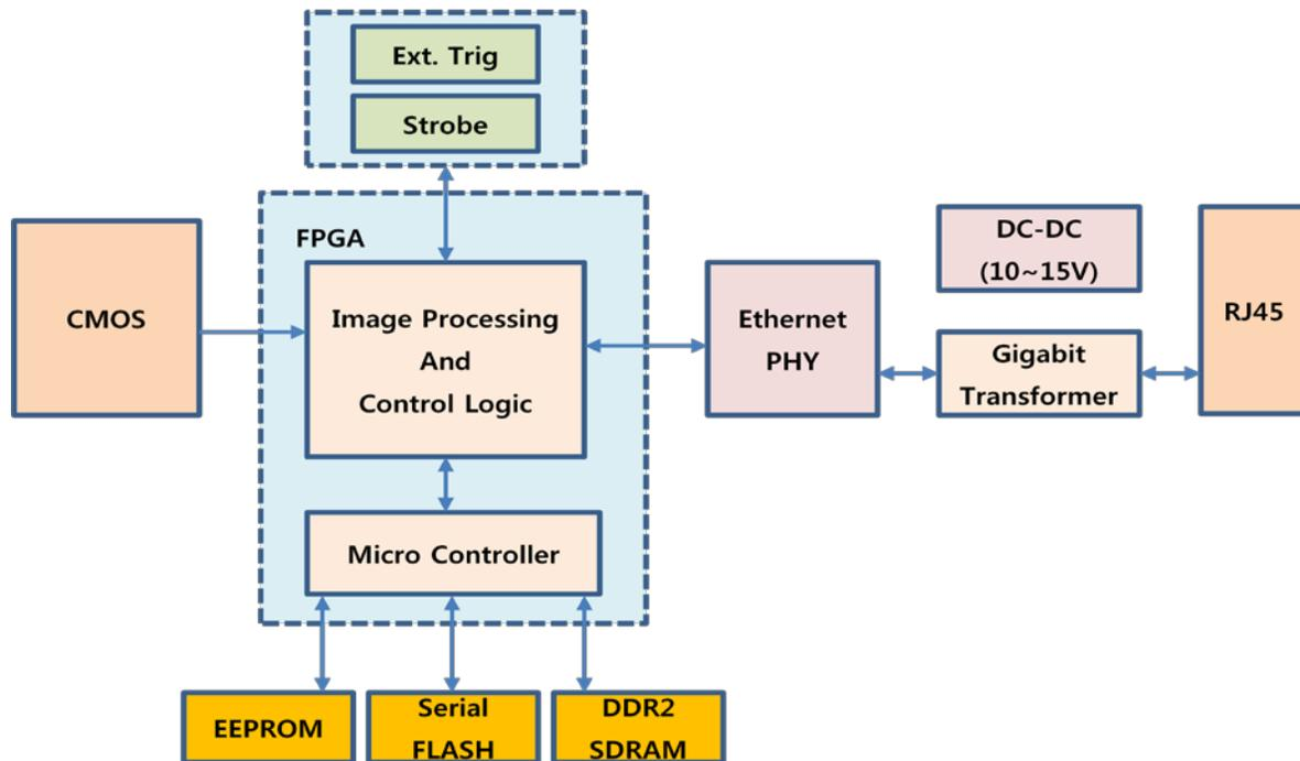
Figure 5.2 Camera Block Diagram (VQ-310G-M400)
