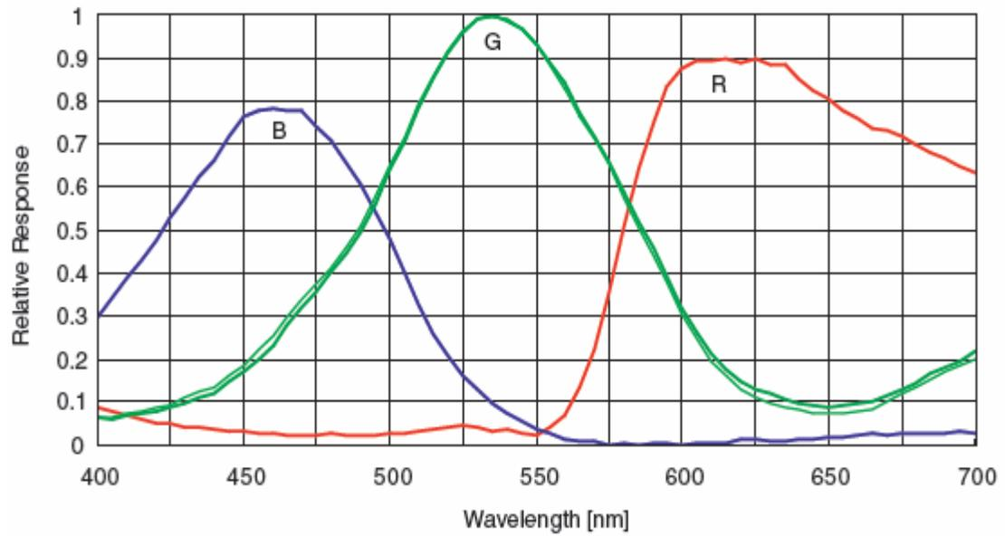
Figure 5.11 VQ-5MG-C16 Spectral Response
