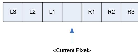
**Figure 10.25 Location of Defective Pixel to Be Corrected**
