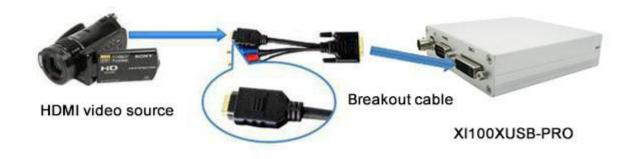
Figure 3, HDMI signal connection sketch map
