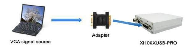
Figure 4, VGA signal connection sketch map
