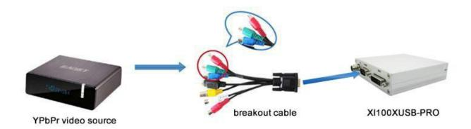
Figure 6, second YpbPr signal connection sketch map
