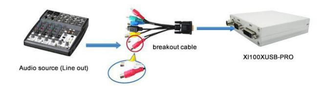
Figure 9, audio line in signal connection sketch map
