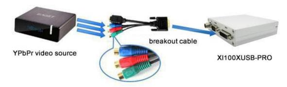
Figure 5, first YpbPr signal connection sketch map
