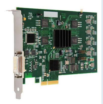
The XtremeDVI-DualLink is a single channel PCI express Dual (or Single)-Link DVI video capture card. A stand alone PCIe x4 plug in card, the XtremeDVI-DualLink delivers extreme performance with 650MB/s transfer bandwidth.
