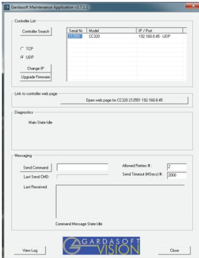
GardasoftMaint allows you to view the controllers on your network, change their IP addresses and Gardasoft can upgrade their firmware if it becomes necessary. In the messaging section of GardasoftMaint, you can communicate with your controller using the commands explained in Section 10, Command configuration. You can also open the selected controller’s web pages at the click of a button. For more information about the CC320’s web pages, see Section 9, “Web page configuration”.
