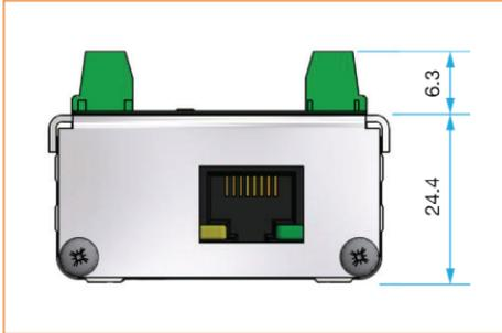
The CC320 does not have an IP rating and should be mounted such that moisture and dirt cannot enter the unit.
