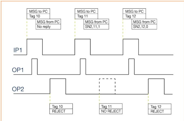
In this example, three product triggers were received. The camera was triggered using OP1.
