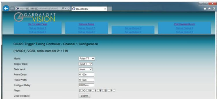
You can set up all the parameters for each output channel. Pressing the Submit button updates the CC320 configuration and saves the changes to non-volatile memory. On this page you can:
