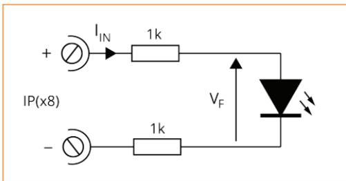
An input voltage between 5V and 24V is recognised by the CC320 as a logic level '1'. An input voltage of 2V or less is recognised as a logic level '0'.
