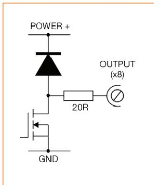
The voltage between the output and ground must not be greater than 24V and the output can only sink up to 50mA.
