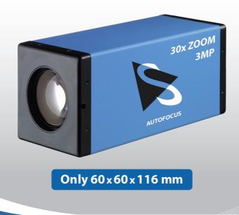
The Imaging Source DFK Z30GP031 color camera has a GigE interface and is the perfect solution for many industrial automation, quality assurance, security, surveillance and medical applications. The color camera ships with the very sensitive 1/2.5 " Aptina CMOS MT9P031 sensor. With up to 22 images per second, the DFK Z30GP031 is a low cost, yet highly versatile imaging solution. The camera integrates an autofocus lens (auto/man).
