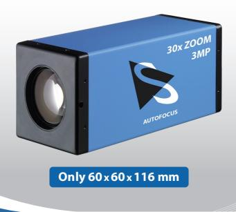
The Imaging Source DMK Z30GP031 monochrome camera has a GigE interface and is the perfect solution for many industrial automation, quality assurance, security, surveillance and medical applications. The monochrome camera ships with the very sensitive 1/2.5 " Aptina CMOS MT9P031 sensor. With up to 22 images per second, the DMK Z30GP031 is a low cost, yet highly versatile imaging solution. The camera integrates an autofocus lens (auto/man).
