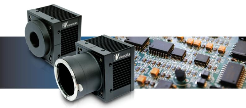
VH series is a Progressive Scan type high-resolution industrial Area Scan camera. All functions can be programmed and updated in the field without any disassembling process. The variety of resolutions from VGA to 5 megapixels provide flexibility and makes the VH series suitable for a wide range of applications such as Machine Vision, Research, Scientific and Remote Sensing applications.
