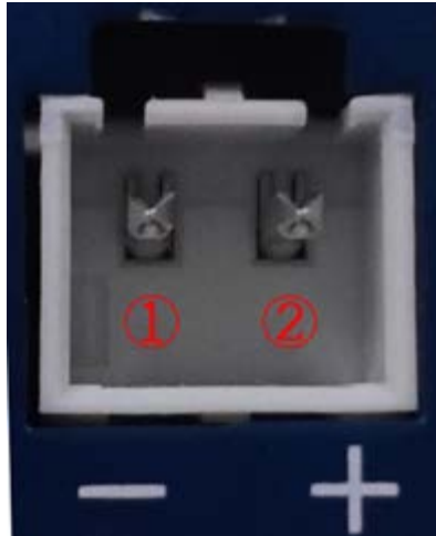
Figure 7.3 Pin Arrangement of Power Input Receptacle
